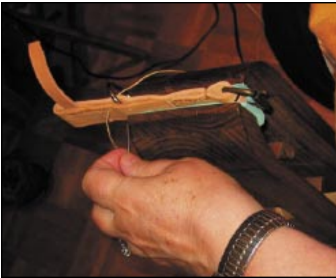
The photo shows the needle being inserted into the pierced hole from the back side of the project.
