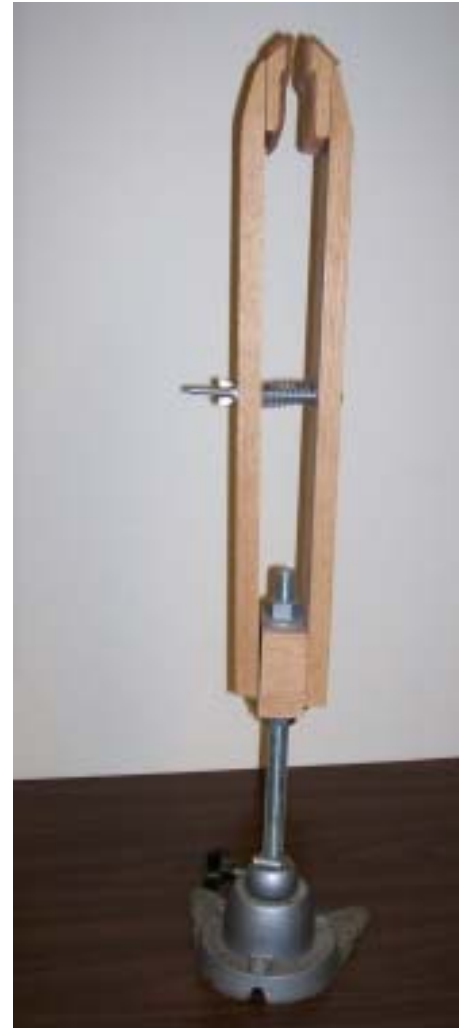
Terry Bowman's Stitching Horse is mounted on a PanaVise base for flexibility.
