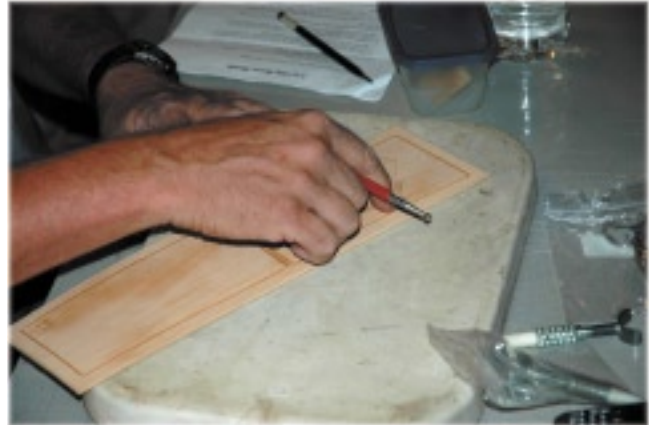
Ball end to round over the swivel cuts
