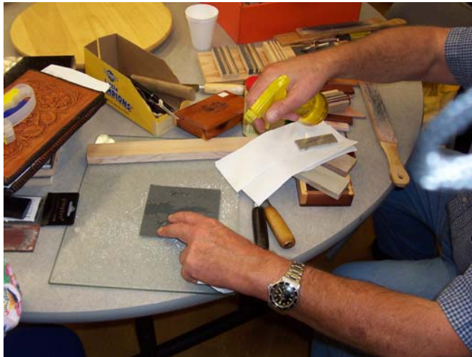
Placing the sanding film on the flat surface and wetting it
