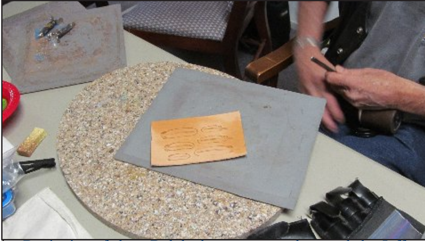
Beginning of class. Bob had us use a template made by Jeff Mosby (Grey Ghost Graphics) to put the pattern on the leather. Made things much simpler.
