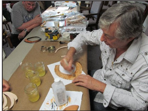
First step in construction is to apply the contact cement to the plug and the top layer.
