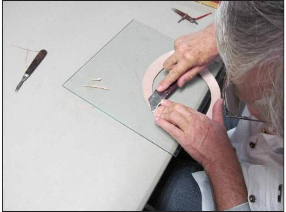
Skiving the middle layer of leather (the plug) to a feather edge.
