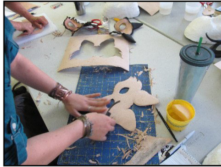
Skivving the outside of the mask to a feather edge makes it easier to form.
