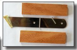
curing the scales are shaped, sanded, and given a coat of finish.
