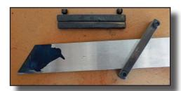
Another line is marked 4 \(^3\)/4 from the tip of the blank, the jig attached, and the bevels ground with the right handed knives beveled on right and the left handed ones on the left.
