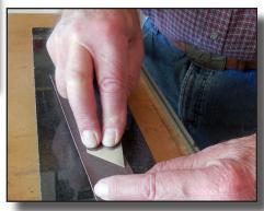
series of sandpapers up through 2500 or by stones. I have used both. Either way, I like to use a King finish stone last, before stropping.
