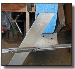
blank is heated to a bright red in the forge and quenched in oil. Very hard but brittle. Some of that hardness has to be drawn off. To do this I use a toaster oven set at 400 and let them soak for 1 hour.
