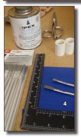
cut a piece of <sup>3</sup>/<sub>4</sub>" PVC pipe into a bunch of 1-1/2" long tubes.
