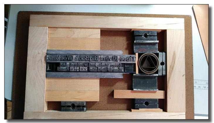
that I constructed by gluing and screwing with construction Torex headed self tapping screws. The initial hole was drilled undersized and the wood glue and screw completed the frame. Since the frame is only 3/4" (0.75") and metal printing type is 0.918" high, only the type gets embossed into the leather. The the construction of the frame is similar to the metal "chase" that printers use using movable type setting, like the old newspapers in the 1800's.
